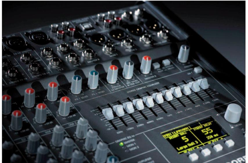
Graphic EQ and display for the internal effects section
